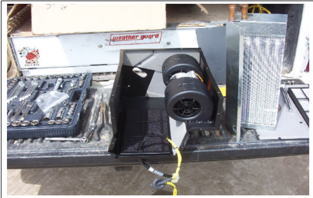
Heater box with heater coil and mount frame removed.
