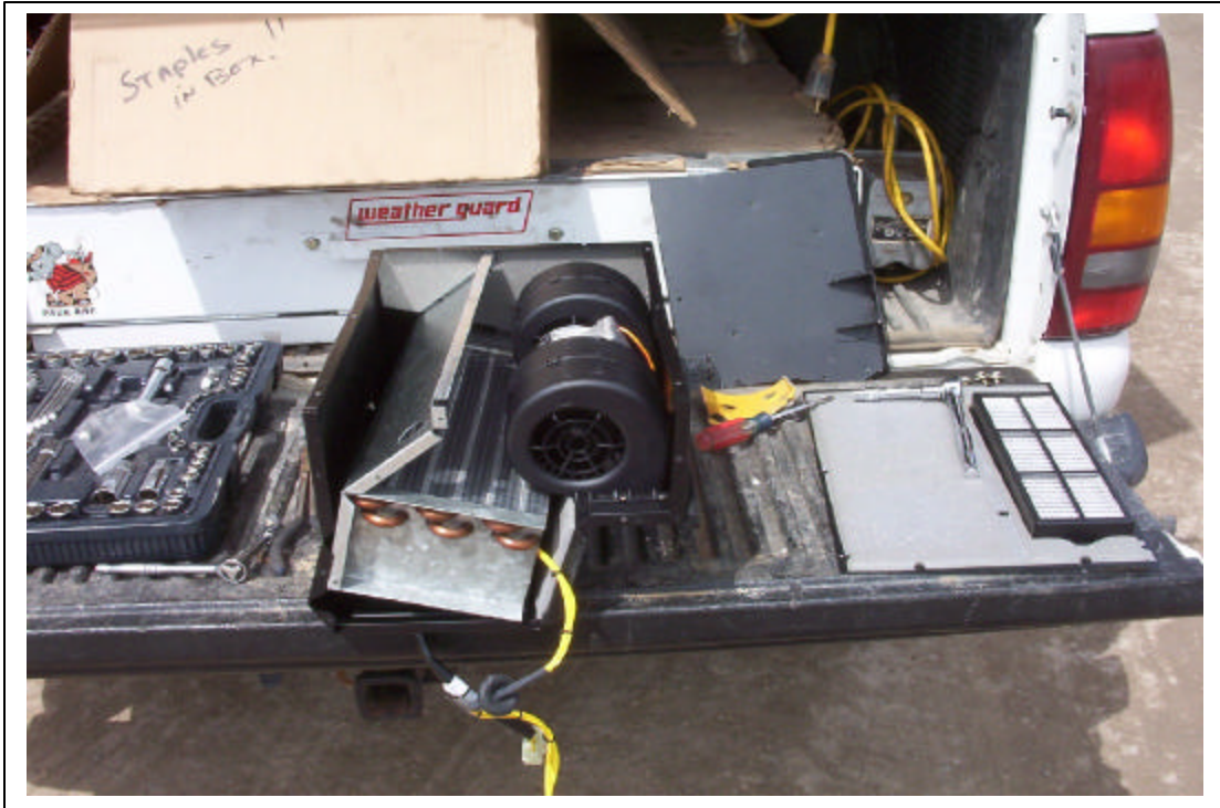
Heater box with the lid and end removed.
