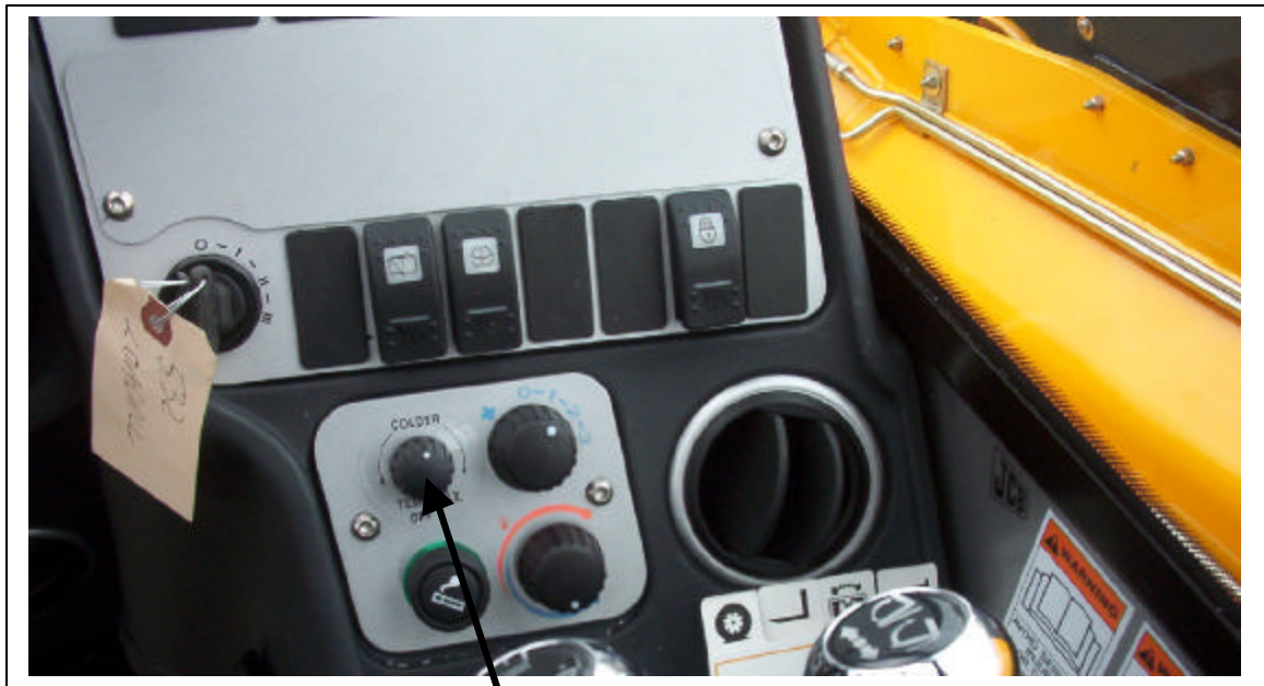
Thermostat and decal installed.
