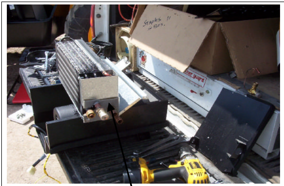
Some metal may have to be removed from the end of the heater frame to allow A/C fittings to fit.
